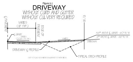
In the case of a street that is planned to hold stormwater in a ditch (in some cases front yards) between driveways. The driveways shall be graded to meet the property line at an elevation of 4.5 inches (for a 60 ft. right of way) or 6 inches (for a 66 ft. right of way) above the centerline of the street pavement. See figure (c.)
