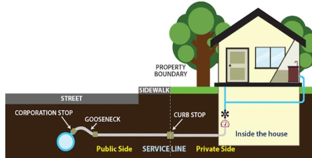
**Image B:** The lead gooseneck is a flexible connection roughly 12 inches in length, that connects the service line to the water main. The city of Stevens Point is proactively removing these over the next three years.
